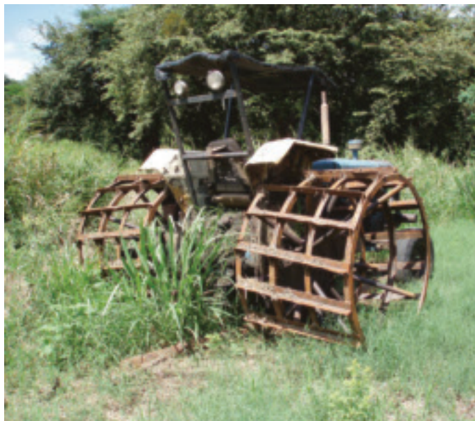
This type of tractor is used by farmers in the wet-rice fields in the Arenal
