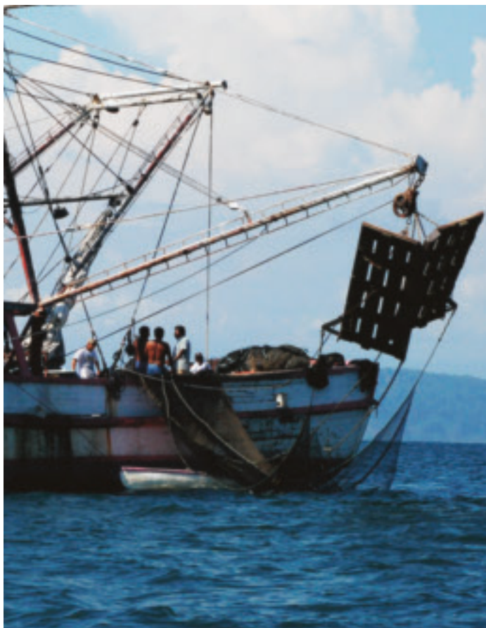
This trawler uses a typical trawl net to catch shrimp from the seafloor.
